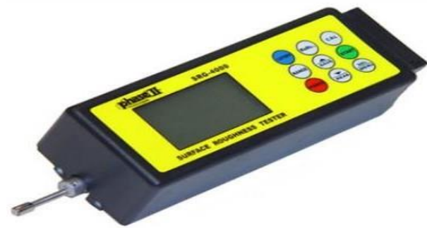
Fig. 2. High-precision stylus profilometer utilized for quantifying the arithmetic mean surface roughness ( R_a ) across the machined evaluation lengths.
