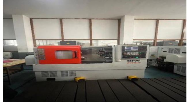
Fig. 1. Experimental setup of the Bharat Fritz Werner (BFW) Orbitur Plus CNC turning center utilized for the machining of EN-31 and Mild Steel workpieces under flood cooling conditions.
