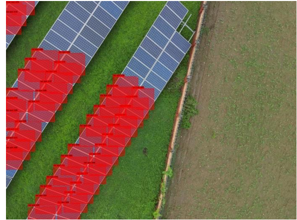
Fig. 4. Mask R-CNN detection at confidence threshold 0.90: 45 detections retained at higher certainty.
