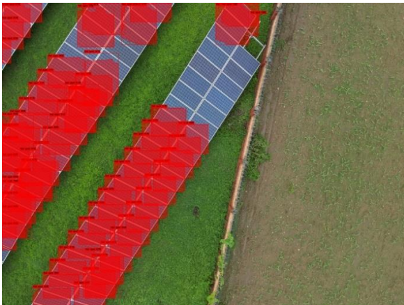
Fig. 3. Mask R-CNN detection at confidence threshold 0.55: 65 hot-spot regions identified with pixel-level instance masks.
