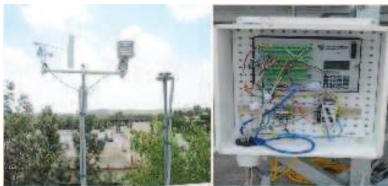
Photo 3: Weather station and CS Campbell Scientific Data-logger
