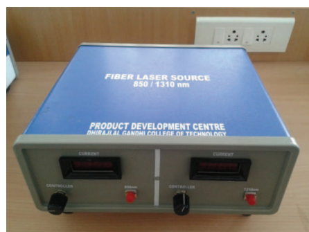
Fig 2. Fiber optic LASER source 850/1310nm
