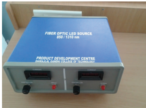
Fig 3. Fiber Optic LED source 850/1310nm
