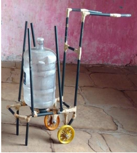
Fig. 3 First prototype of the water carrying contraption
