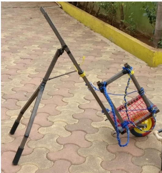
Fig. 4 Final prototype of water carrying trolley
