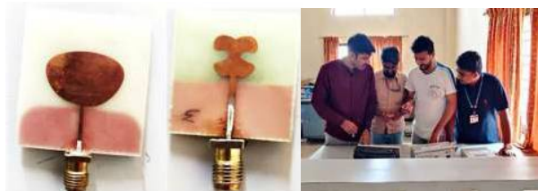
Fig. 5 : Fabricated antennas (left) and Students presenting the fabricated antenna (right)
