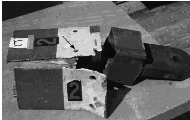
Figure 7: Failure of a hitch due to poor design or overloading conditions
