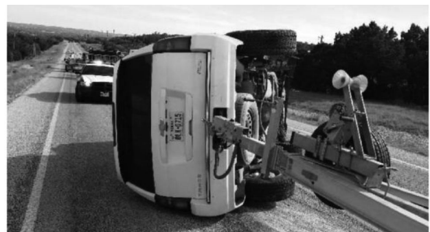
Figure 7: Failure of a hitch due to poor design or overloading conditions
