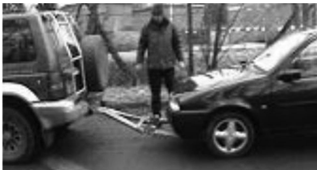
Figure 6: Real life application an axially-loaded tow bar of an automobile [18]
