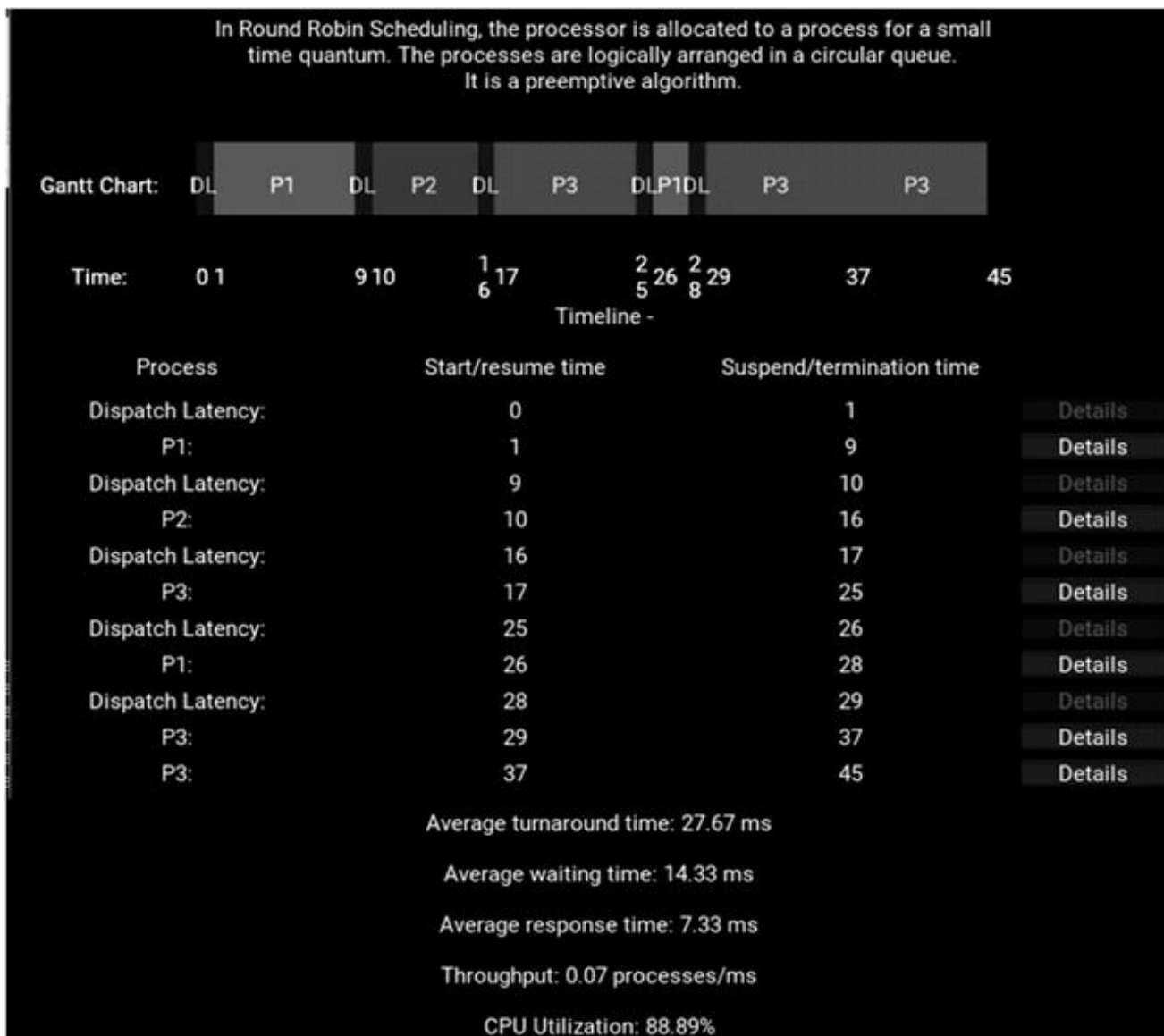
Fig. 1. Sample output of the module to visualize CPU scheduling algorithms. visualizing round robin scheduling with a time quantum of 8 ms and dispatch latency of 1 ms.
