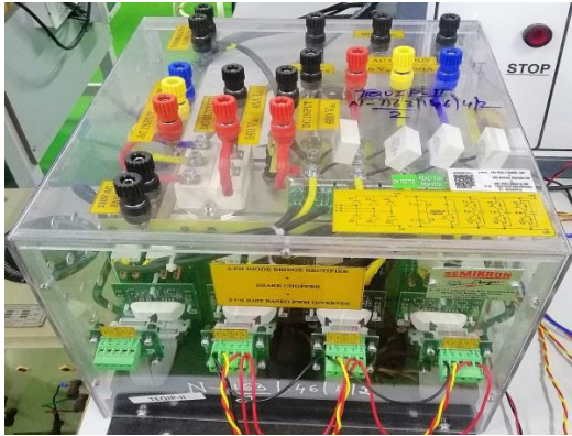
Fig.4 Power modulator block
