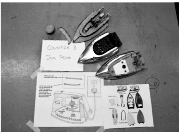
Figure3: Demonstrates construction of Electric Iron consisting of bimetallic strip and Thermostat.
