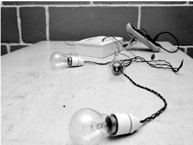
Figure1: Series and Parallel connection: Demonstrating effects of differing wiring schemes on bulb intensity
