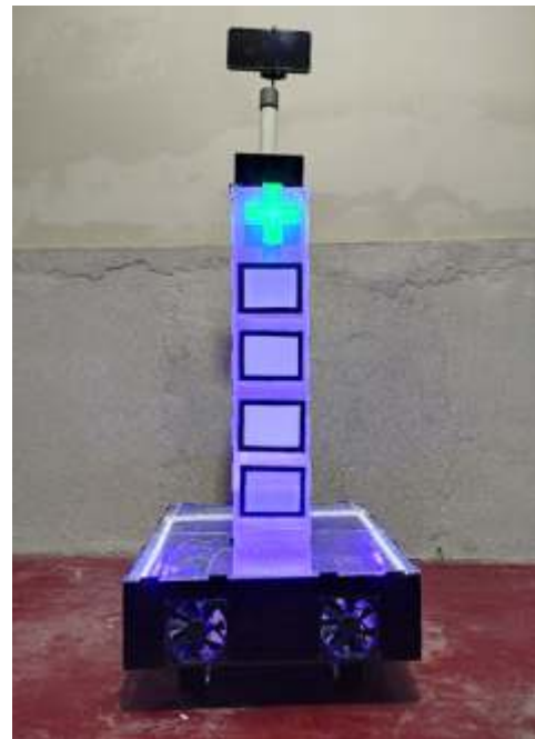
Fig. 9: Working model of an IoT virtual doctor robot
