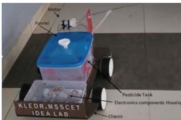
Fig.3 : Working Prototype model of Agriculture Pesticide spraying Robot
