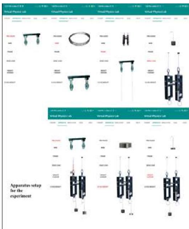
Fig. 4 : Screenshots of a complete experimental setup for computing Young's Modulus of elasticity using Searles' apparatus
