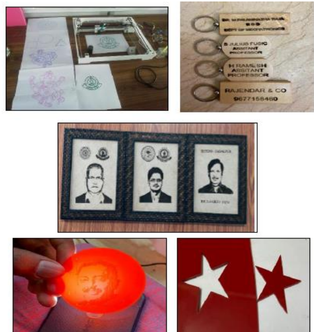
Fig 11: Plotted design, Wood engraved model, Wood engraved design at high precision, Acrylic engrave model, 2mm acrylic board cut model.
