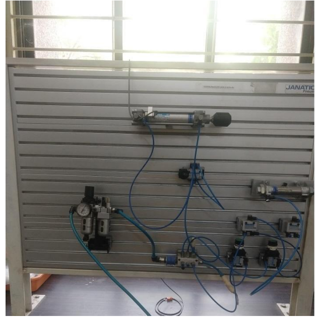
Fig. 6 Demo based group activity: circuit prepared by students on pneumatic trainer kit
