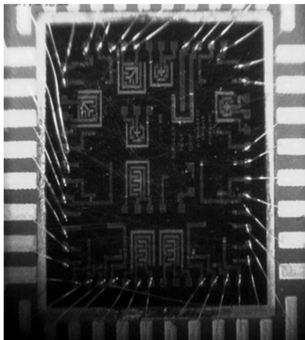
**Fig. 4. MDC wire bonded to ceramic header**
