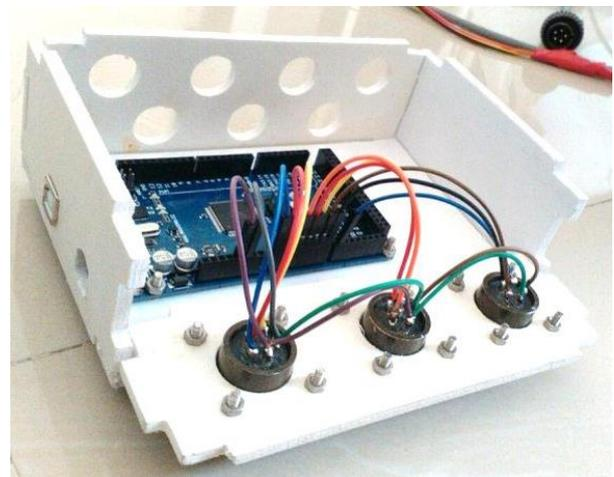
Figure 2: Prototype with three channels for accelerometer
