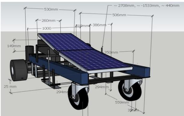
Fig.7Solar powered grass cutter design
