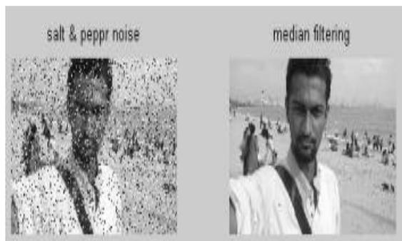
**Fig-4: Median filtering**
