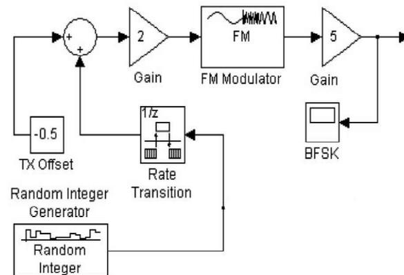
Fig. 5. Implementation of BFSK using simulink tool
