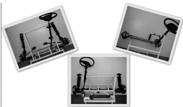
**Fig.5 Cut Section Model of Steering System**
