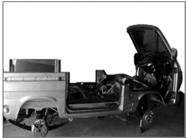
**Fig 2. Cut-Section Model of Chassis**
