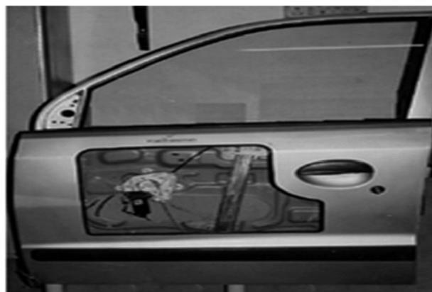
**Fig.3 Cut Section Model of Power Windows**
