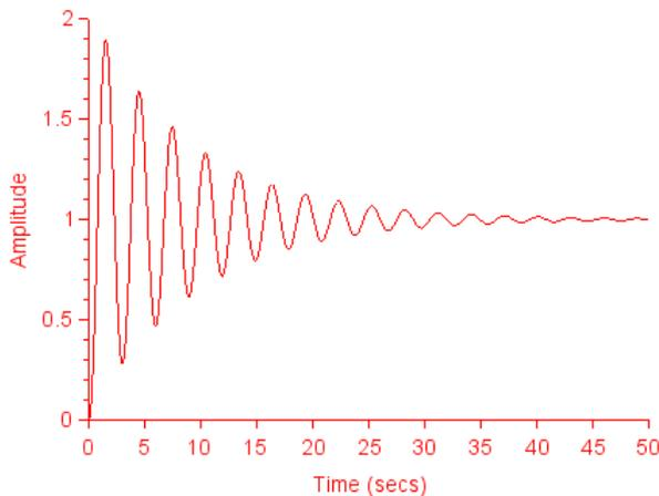
Fig. 8 System response with PI – Controller
