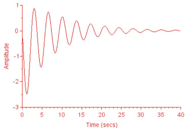
Fig. 4 System response with PI – Controller
