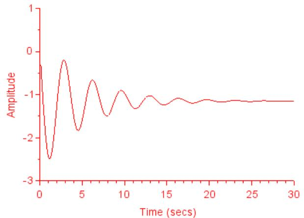
Fig. 3 System response with P – Controller
